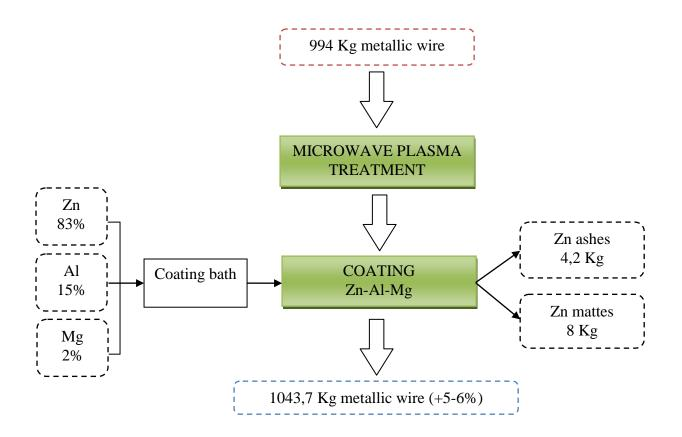
The treatment implemented, as shown in the above analysis, is able to minimize the components entering in the system and those exiting from the system itself. In the case of waste products, these are reused in the system itself or in other treatments. The only products that have to be disposed of are the Zn mattes and ashes which are produced in a lower quantity if compared to the traditional systems since the new coating system operates at lower temperatures.
