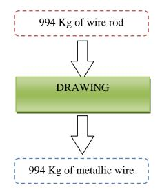
Once the wire rod has been cleaned and drawned, the metallic wire undergoes the plasma-microwave treatment instead of the conventional treatment with ammonium chloride. Such treatment has the double objective of removing the impurities still
