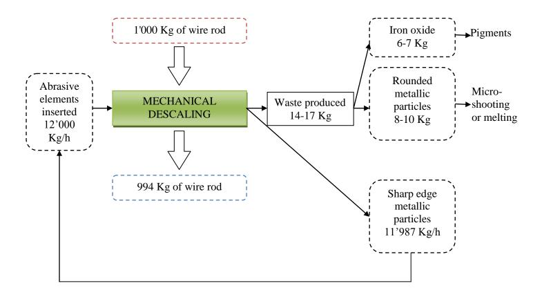
As can be easily seen observing the figure above, the entering wire rod (1'000 Kg), is hit constantly by the abrasive material aiming at cleaning the surface of the products. This process determines the detachment of impurities from the wire rod, aspect which determine a lower weight of the product when exiting from the system (around 0,6-0,7% less).
