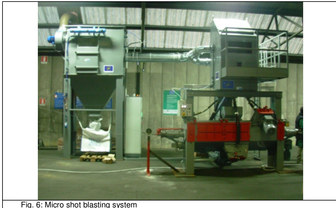
Fig. 6: Micro shot blasting system
