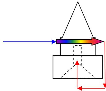
The new geometry of the torch is shown in the figure which also shows an untapered area between the two cones where the entrance and exit of the wire occurs:
