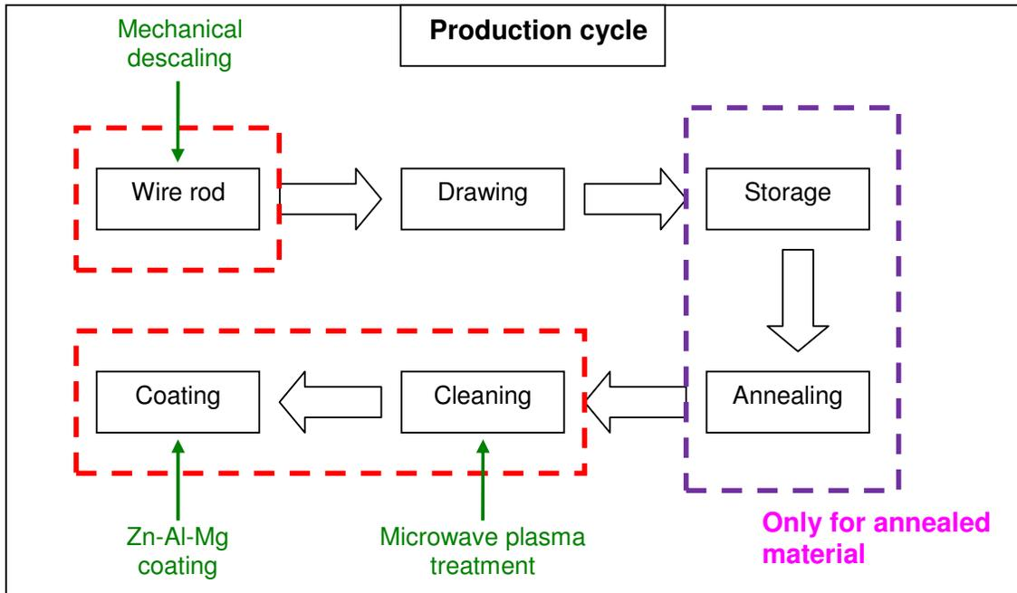
Once the system had been entirely assembled various tests were carried out to check the actual production capacity of the system and the quality of the product obtained. The system can treat 1000 Kg/h of wire as foreseen and the output product features excellent characteristics in terms of mechanical and corrosion resistance.
