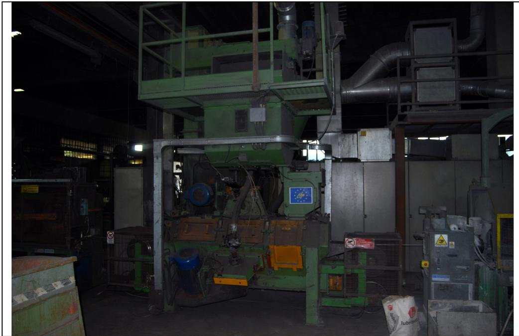
Photo 1: Mechanical descaling system
