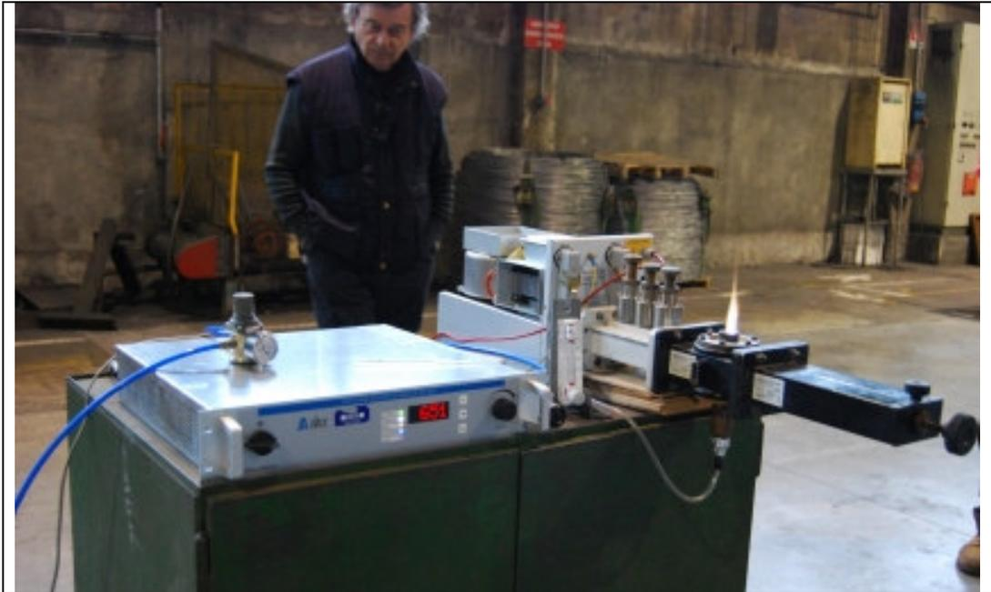
Photo 2: First prototype of microwave plasma torch
