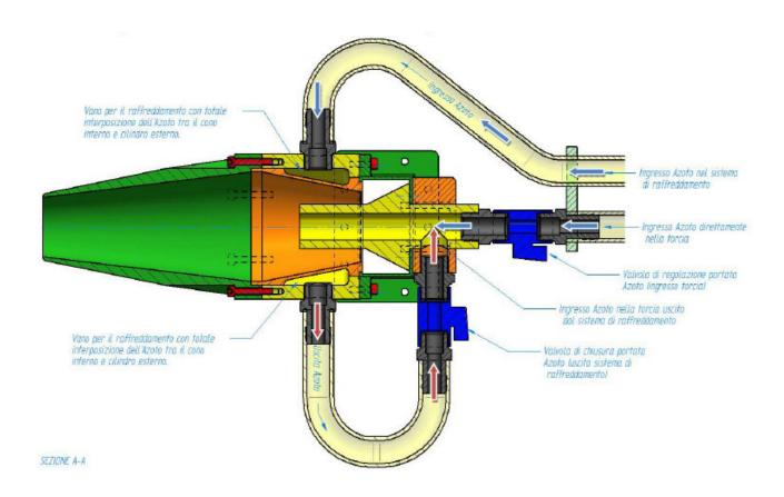
The wire to be treated passes at the end of the nozzle (yellow), which creates the plasmatic flame.
