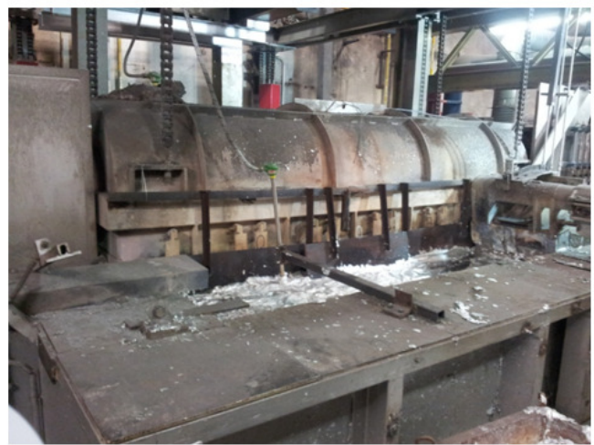
Dip coating system – Zn-Al-Mg
